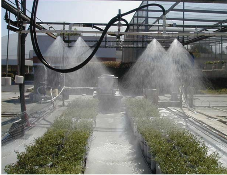
Figure 2. Operating rain simulator. Photo taken in August 2004 while conducting cropped soil experiment.
