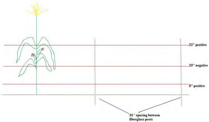
Figure 1. Portable/temporary electric fence design to deter grizzly bear access to Pondera Colony silage cornfields.
