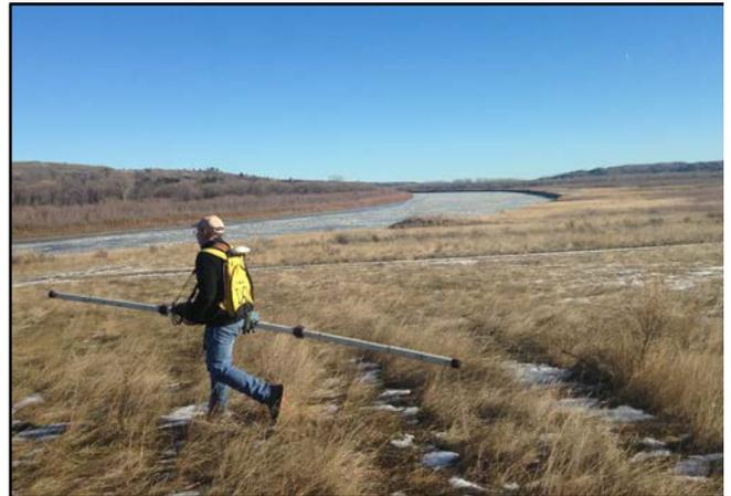
Using Electromagnetic Survey technology to locate buried arsenic bait along Missouri River.
