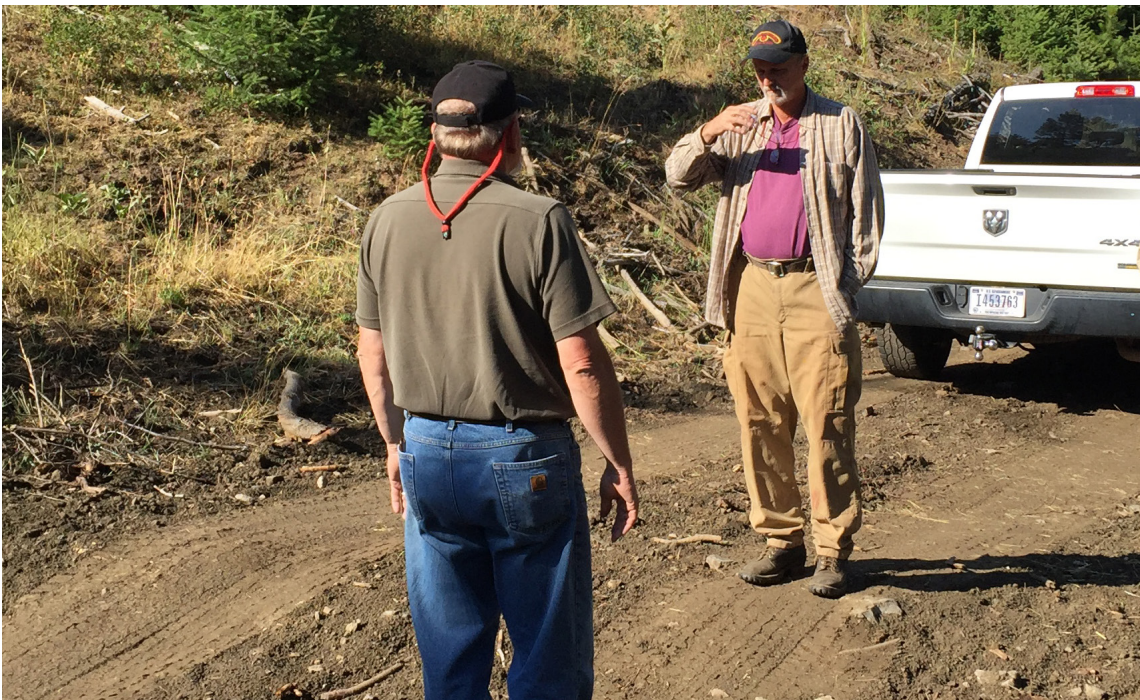
Don Kasten, a forester with the Bureau of Indian Affairs, has Roger Ziesak, the forest practices program manager for the Department of Natural Resources and Conservation, stand in a dip in the road so Kasten can measure the depth. Road dips help slow down water runoff and prevent sediment from reaching streams.
