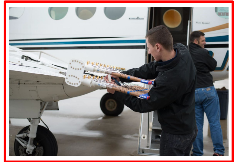
Wing mounted "Burn-in-Place" (BIP) flares
