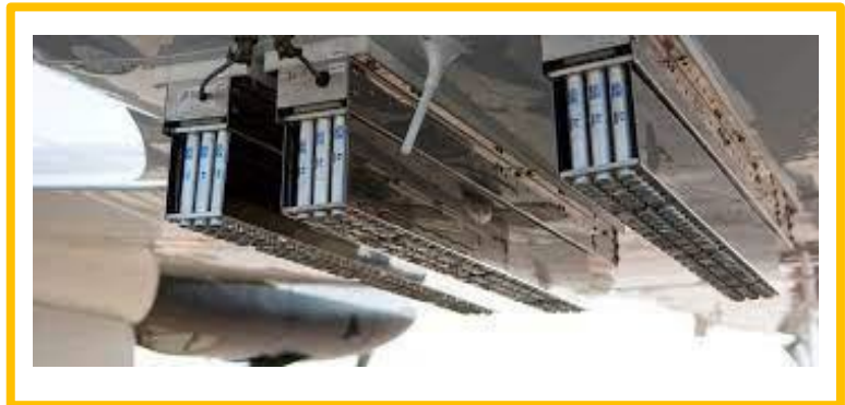
Belly Mounted Ejectable (EJ) flares
