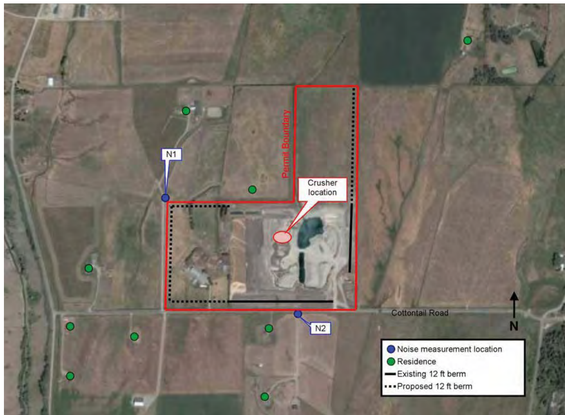
Figure 5. Ambient noise measurement locations near the Nuss-Rock pit near Gallatin Gateway, Montana.
